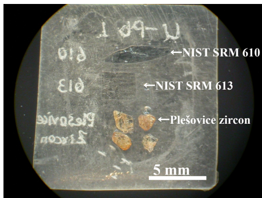
Fig. 1. Plešovice zircons and NIST SRM 610, 613 glasses mounted in an epoxy resin.
